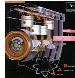
Integrated Starter Alternator Damper
